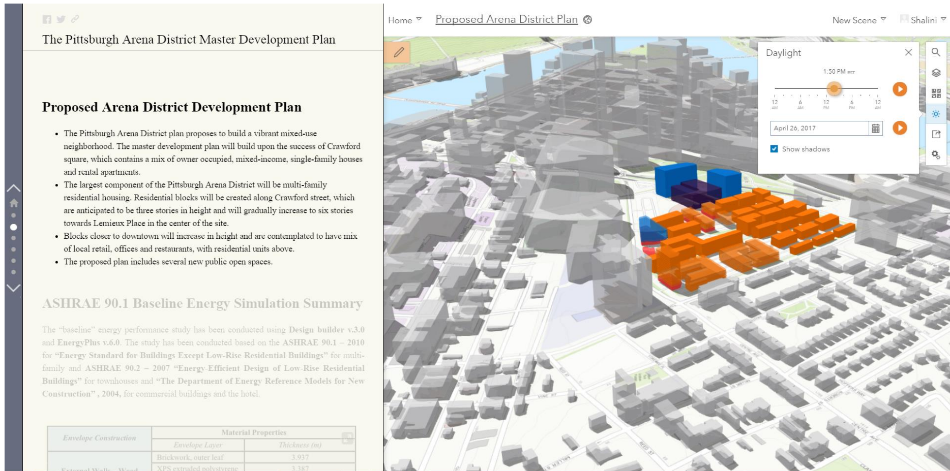
Figure 68. Story map provides daylight and shadow analysis for the Lower Hill District
