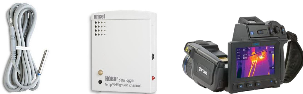
Figure 21. Equipments used to measure air and façade temperature
